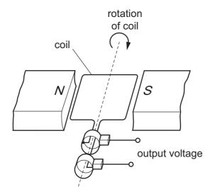
As the coil passes through the position shown, the output voltage is +10V.
